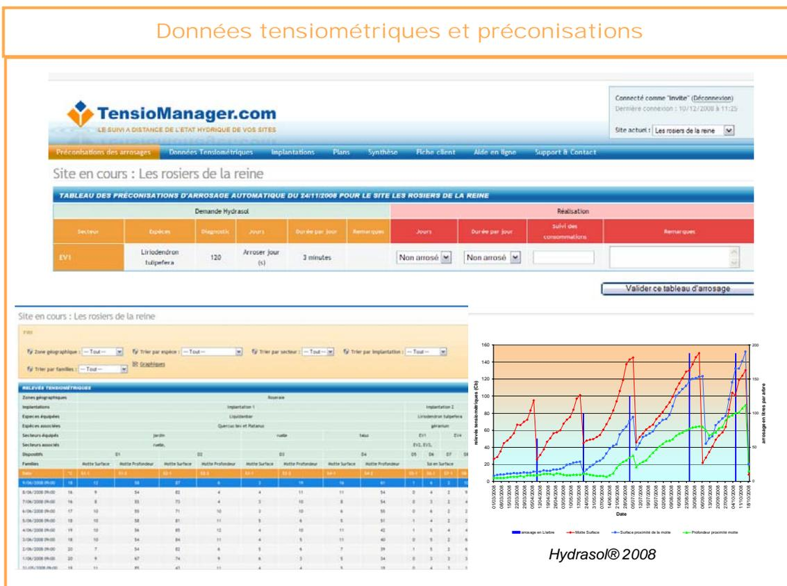
The screenshot displays the TensioManager.com interface for the site 'Les rosiers de la reine'. It includes a navigation menu, a 'Demande Hydrasol' table, and a 'RELEVÉS TENSIO MÉTRIQUES' table. A graph on the right shows soil moisture levels (Cv) over time for different sensor locations.
